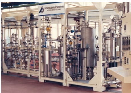
First pilot plant - supercritical fluid extraction
