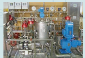
Particle generation plant up to 80 kg/h, up to 350 bar
