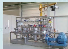
Supercritical fluid extraction R&D unit, 5 l/1000 bar
